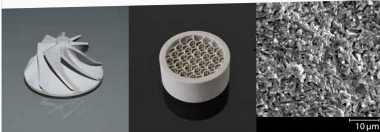
Silicon nitride is a beta-SiAlON type ceramic. It exhibits superior material properties such as high strength, high toughness, thermal shock resistance and good chemical resistance to corrosion from many acids and alkalis.
