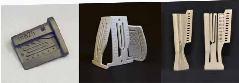
LithaCore 450 is mainly based on silica with addition of alumina and zircon. It is used for the production of casting cores for investment casting. Typical applications include single crystal casting of turbine blades.
