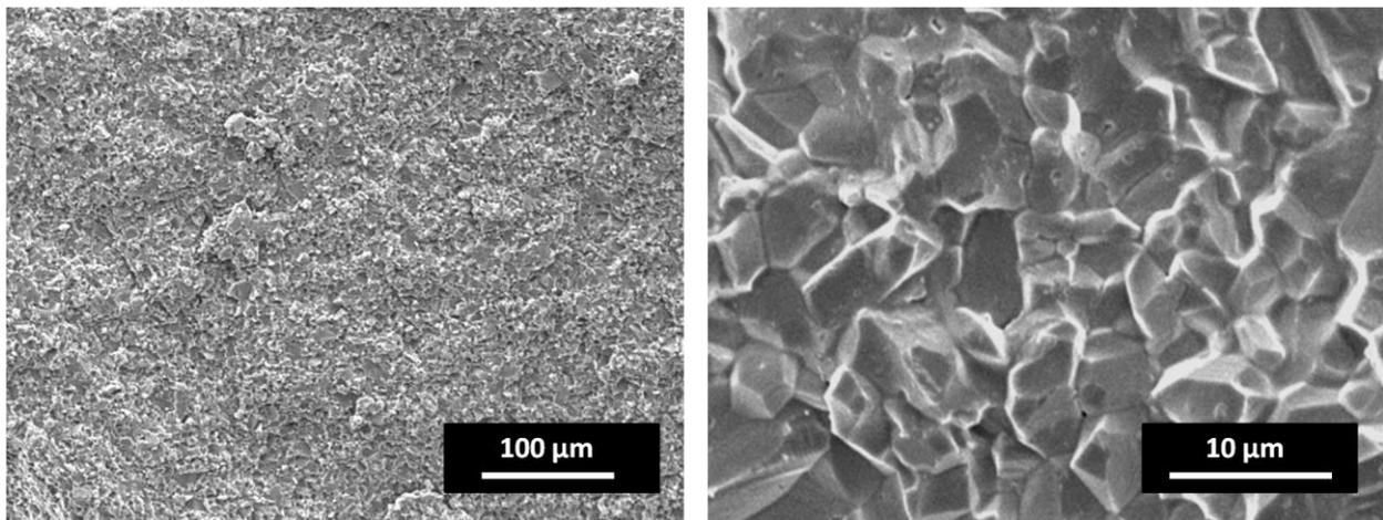
**Fig. 3** Fracture surfaces of a 4-point-bending test bar
