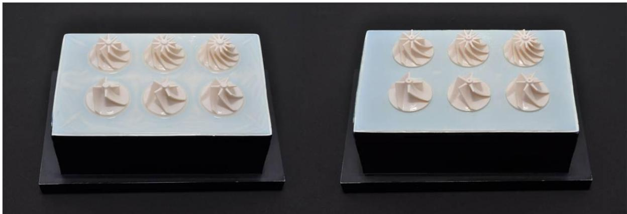
**Fig. 1** Building platform of the CeraFab 7500-system with structured green parts: left – uncleaned parts directly after building process; right – green parts cleaned in an adequate cleaning fluid
