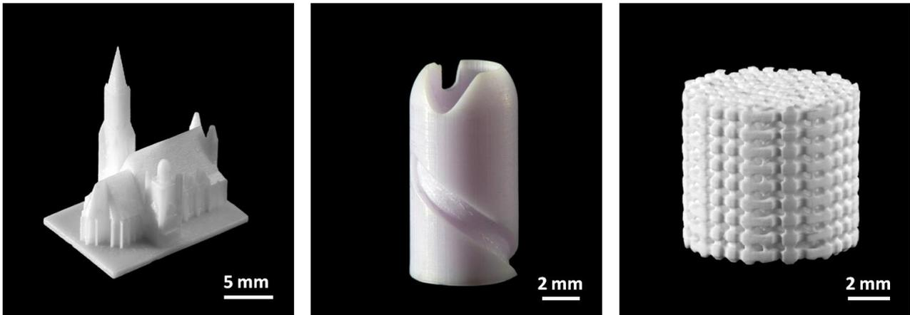
**Fig. 2** Sintered ceramic parts made from the three standard materials currently available at Lithoz: left – St. Stephen’s cathedral in Vienna at a scale of approximately 1 : 6500 made from LithaLox HP 500 ( $\text{Al}_2\text{O}_3$ ); middle – hull made from LithaCon 3Y 610 Purple (TZP); right – cellular scaffold made from LithaBone TCP 200 (TCP)
