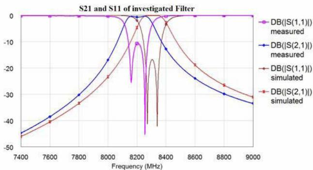
Figure 2. Comparison of measured and simulated S-parameters
