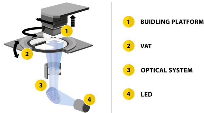
*Fig. 2. System employed to manufacture the green body.*
