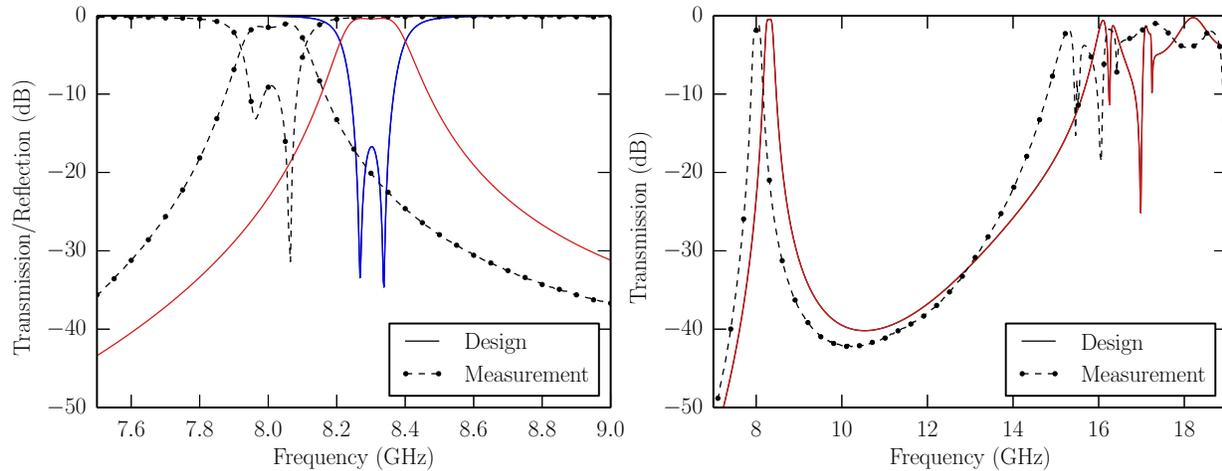
**Fig. 7.** Measured response of the filter shown in Fig. 6 compared with design performance.
