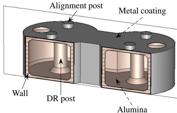
**Fig. 1.** View of the proposed two-cavity monoblock ceramic filter.
