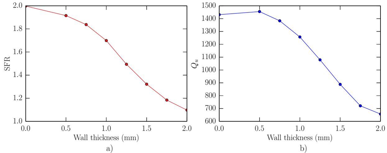
**Fig. 4.** Effect of the wall thickness on the resonator performance. Central post radius has been adjusted to ensure that the fundamental mode resonates at 8.3 GHz.
