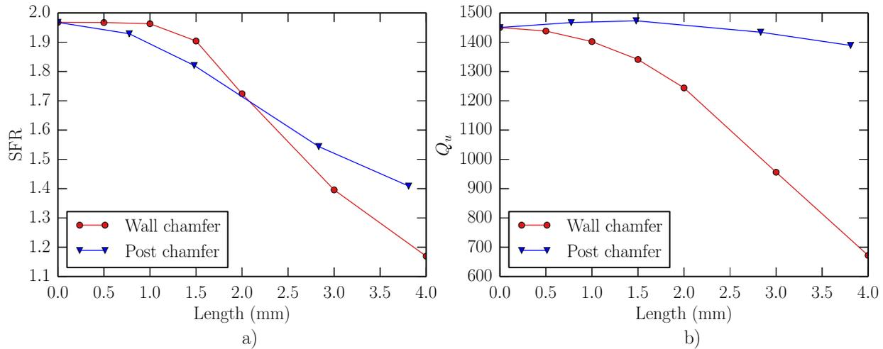
**Fig. 5.** Effect of the chamfer length (at the post-wall junctions as well as wall-wall junctions) on the resonator performance. Central post radius has been adjusted to ensure that the fundamental mode resonates at 8.3 GHz. Simulations have been performed with a wall thickness of 0.5 mm.
