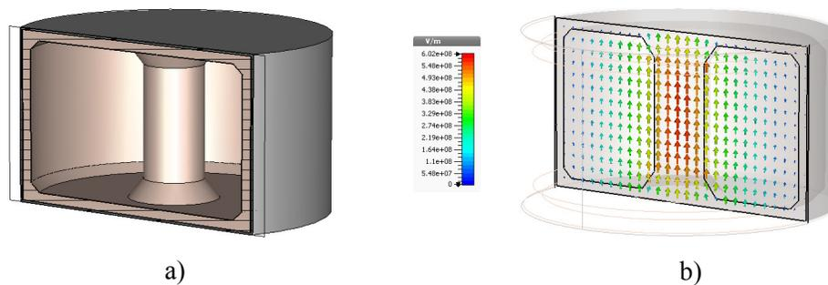
**Fig. 3.** Single ceramic cavity.
