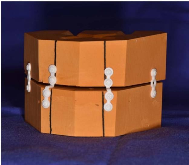
Fig. 1. The experimental set up showing the two cast blocks, reflecting the separated maxillary segments stabilized in the desired position using virtually planned and individual fabricated ZrO<sub>2</sub> mini-plates.
