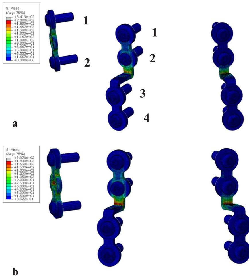
Fig. 4. (a) Three-dimensional highest Von Mises stress locations occurring in model I on the titanium screws (numbered from top to bottom) and plates. (b) Three-dimensional highest Von Mises stress locations on ZrO<sub>2</sub> screws and plates (model II) under 500 N of loading.
