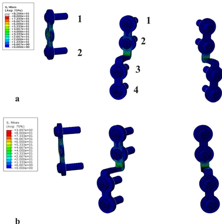
Fig. 3. (a) Three-dimensional highest Von Mises stress locations occurring in model I on the titanium screws (numbered from top to bottom) and plates. (b) Three-dimensional highest Von Mises stress locations on ZrO<sub>2</sub> screws and miniplates (model II) under 120 N of loading.
