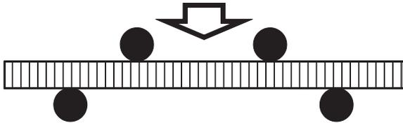
Fig. 5. Schematic set-up for 4PB testing to clarify the orientation of the individual layers.
