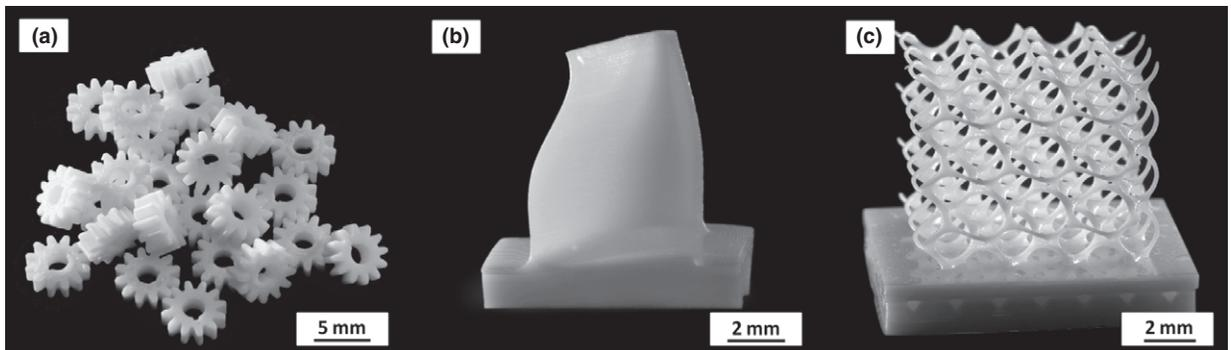
Fig. 7. Sintered alumina parts fabricated using the LCM technique: (a) gear wheels; (b) a turbine blade; and (c) a cellular cube.
