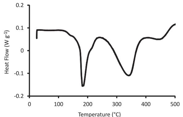
Fig. 4. DSC measurement of the alumina green part.
