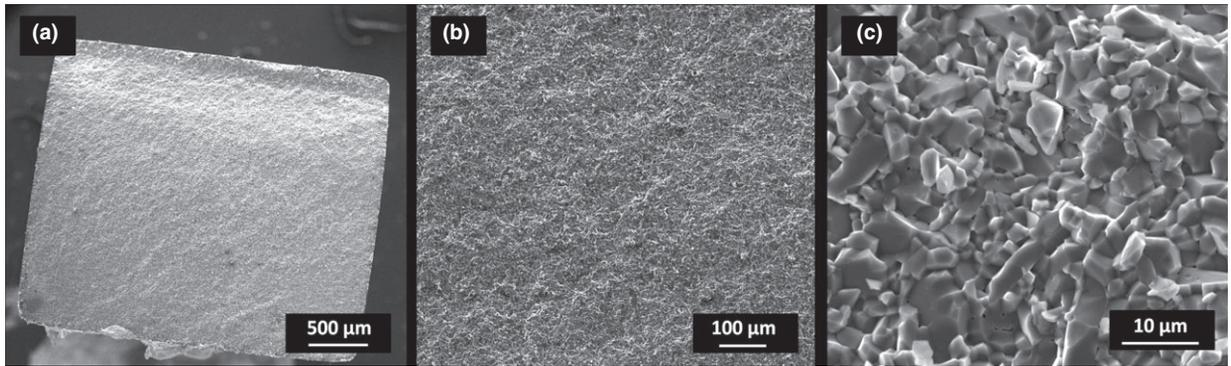
Fig. 8. SEM micrographs of the 4PB fracture surfaces of the sintered alumina specimens in different magnifications.
