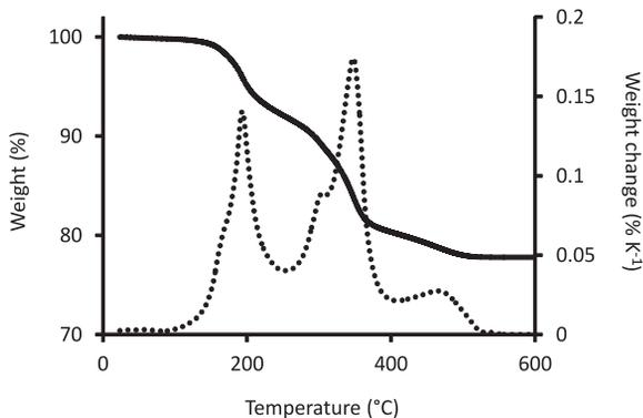
Fig. 3. TGA measurement of the alumina green part: weight (solid line) and weight change (dotted line).
