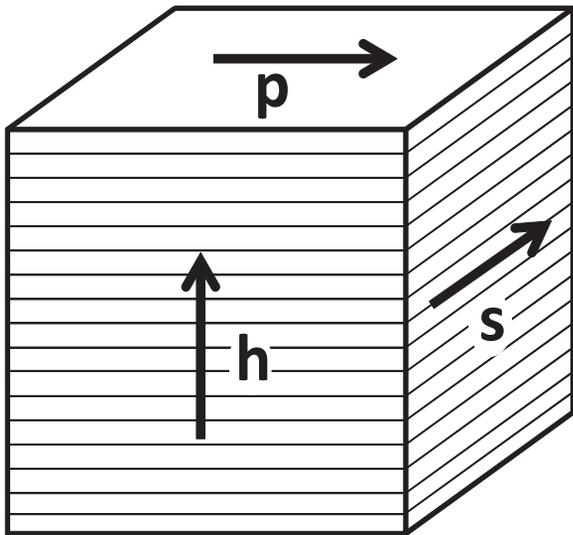
Fig. 6. Schematic drawing for roughness measurements to clarify the orientation of the individual layers.
