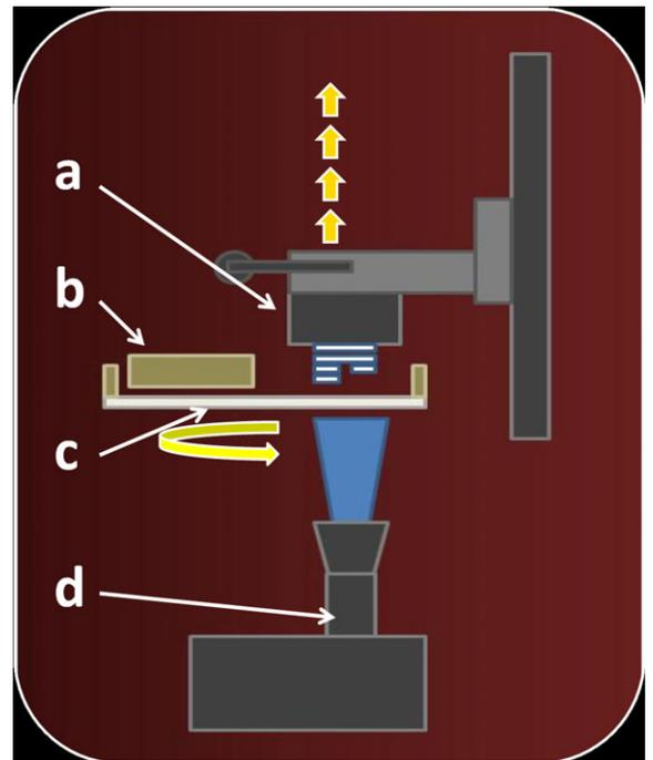
Fig. 1. Schematic drawing of the LCM process: (a) building platform; (b) wiper blade; (c) vat; (d) light engine.
