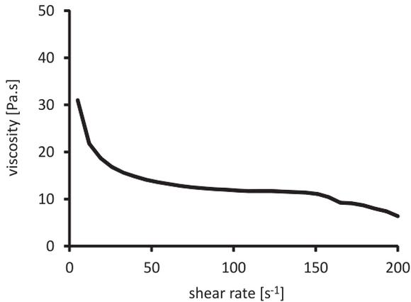
Fig. 2. Viscosity of the photocurable alumina suspension as a function of the shear rate.
