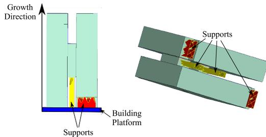
Fig. 4. Orientation of the dual-mode filter during the LCM process.
