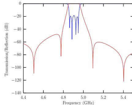
Fig. 3. Ideal S-parameter response of the dual-mode filter
