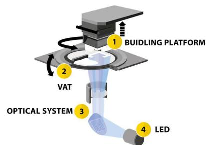
Fig. 1. LCM system employed to manufacture the green body.
