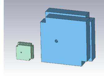
Fig. 2. Size of a TM dual-mode filter implemented with alumina (left) and its equivalent air-filled version (right).
