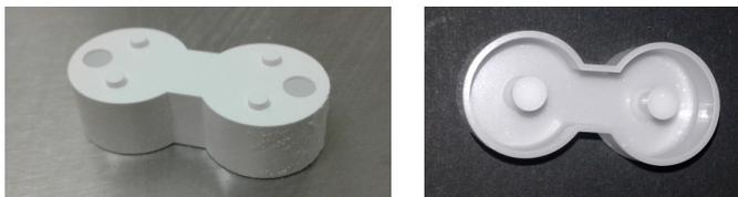
Fig. 6. Left: TM filter manufactured with LCM in alumina. Right: Sample manufactured without the top cover to display the inner part of the filter.
