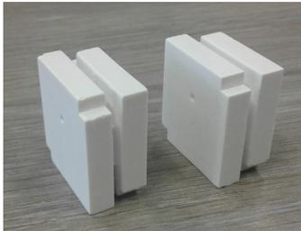
Fig. 5. Two samples of the TM dual-mode filter manufactured as a single part by LCM.
