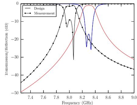
Fig. 7. Measured response of the TM DR filter, compared with design.
