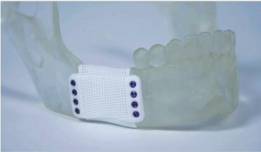
3D-printed ceramics can supply a replacement for bone graft and support structures. This proof-of-concept example from Lithoz actually combines both, with a bioresorbable bone scaffold inside and a stiff outer cage for stability.
