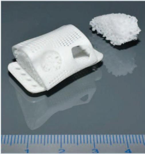
The jaw implant example is a dual-material implant that combines a zirconia cage for stability plus tricalcium phosphate bone graft inserts. The different materials are printed separately and then assembled together. Photo: Lithoz
