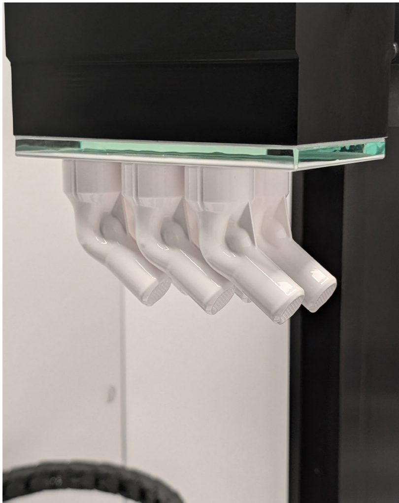
Fig. 2 Six injectors on the LCM build platform after a build (Courtesy Bosch Advanced Ceramics)
