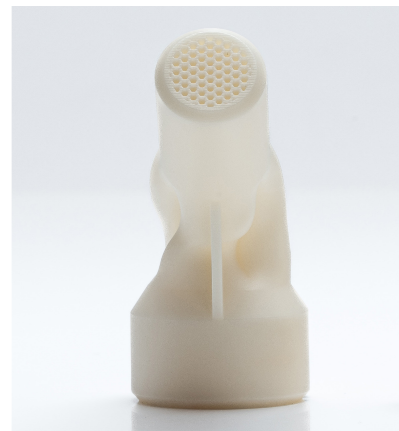
Fig. 1 Ceramic gas injector produced by Lithoz's Lithography-based Ceramic Manufacturing (LCM) process, with three internal channels and sixty-two flow-optimised outlets (Courtesy Lithoz)
