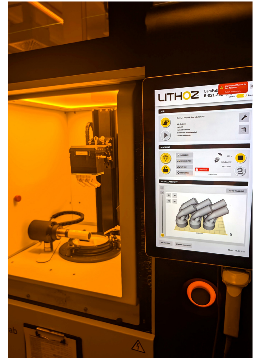
Fig. 5 Injectors in the Lithoz CeraFab machine after a build (Courtesy Bosch Advanced Ceramics)
