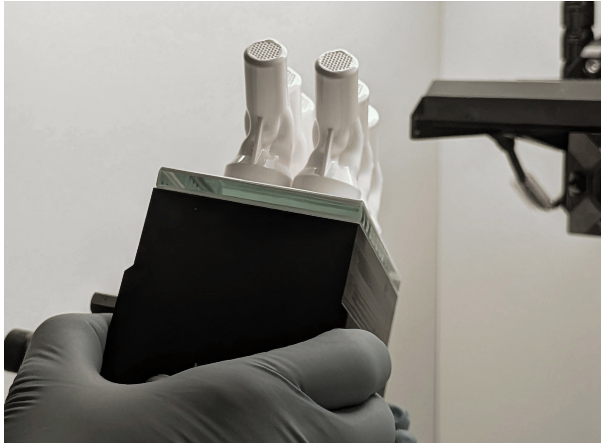
Fig. 6 An operator removing the build from the CeraFab machine (Courtesy Bosch Advanced Ceramics)
