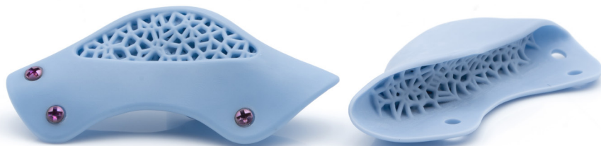
Mandibular angle implant with porous inner structure made of hydroxyapatite material LithaBone HA 480. Left image shows titanium screws for fixation and part of the dense hull has been removed to reveal the inner trabecular-like structure. Right image shows the bone-facing inner structure with defined interconnected porosity and the screw-holes through which the implant is fixed within the defect.
