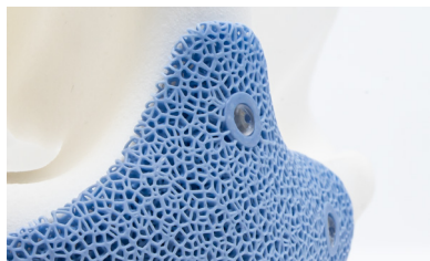
Zygomatic onlay graft made of LithaBone HA 480 fixed with a polymeric, resorbable pin.
