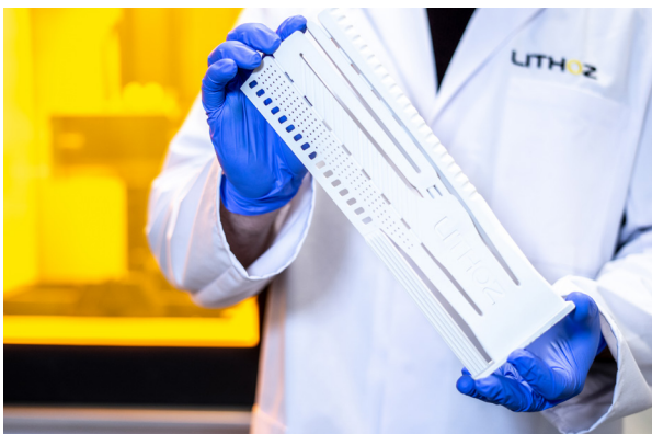
Casting core printed from silica-based ceramic, h = 500 mm
